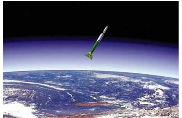
This artist's rendering shows the HyShot hypersonic test payload, attached to its booster rocket, leaving the Earth's atmosphere. Photo: University of Queensland
