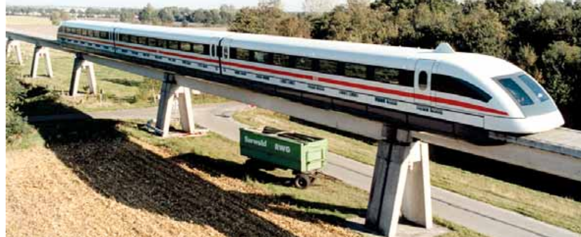
The future of world transportation—magnetically levitated trains capable of travelling at 550 km/hour.
